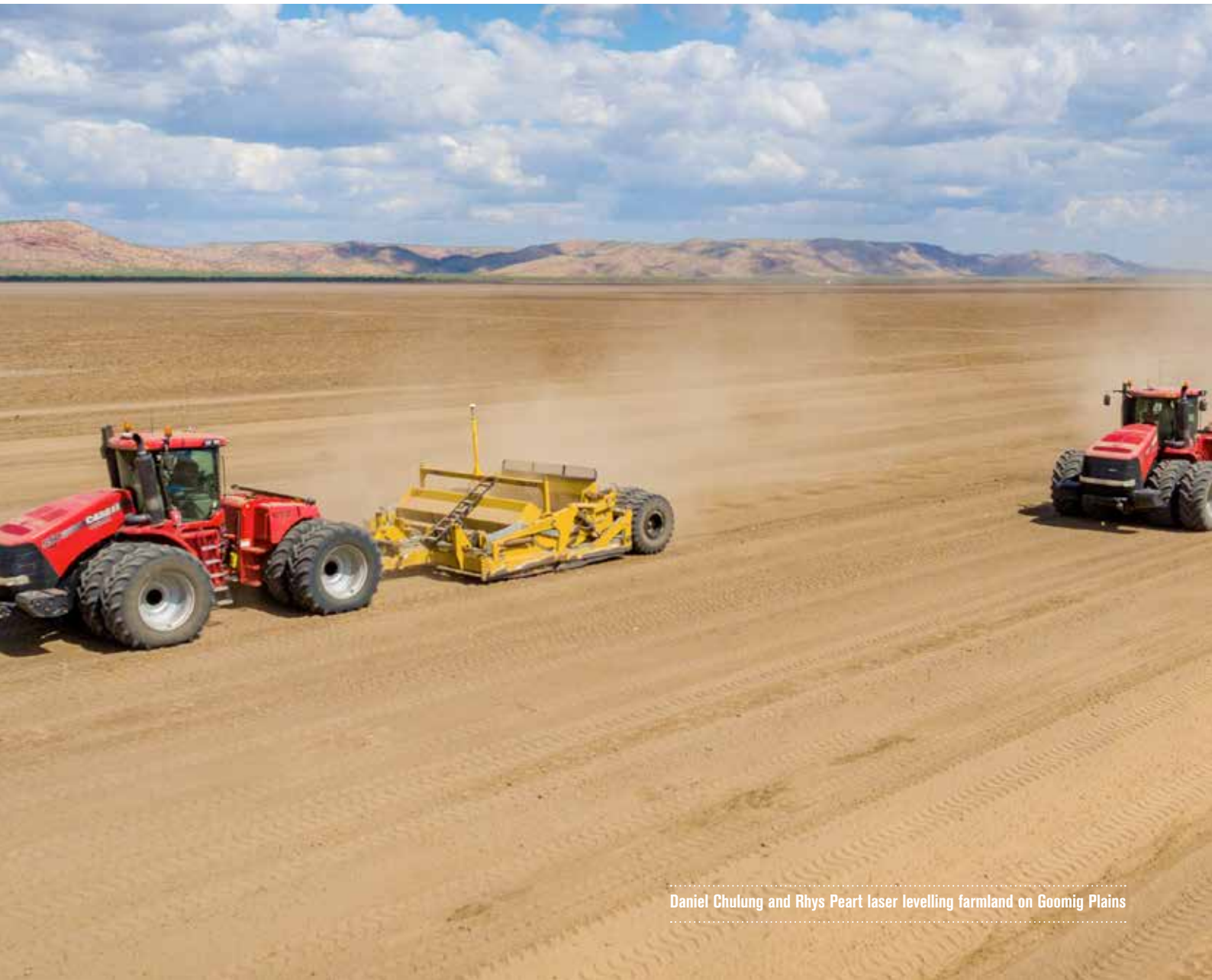
Rhys Peart in the cab of one of the Case 550 Steiger tractors during laser levelling farmland.
